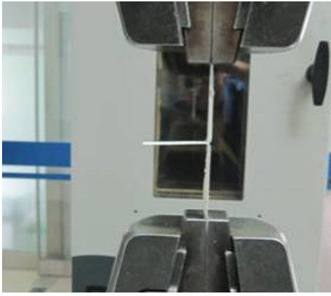
Figure 4: Peel strength testing of test samples joined by the sealant
