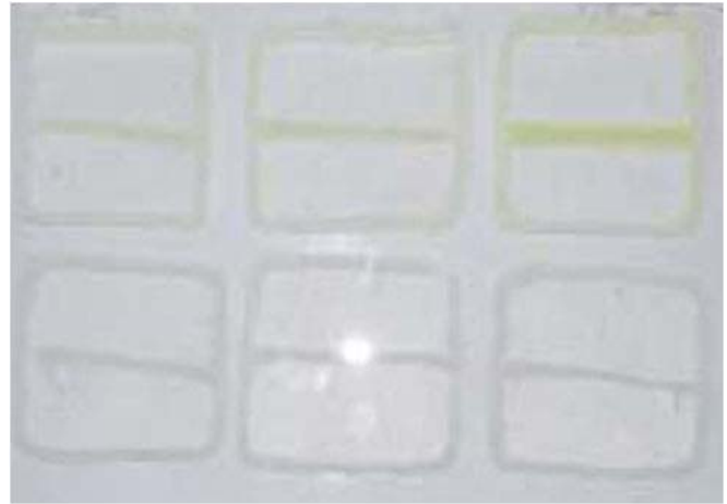
Figure 3: Evaluation of De-oxime Sealant E (Top row) versus De-alcohol Sealant A (Bottom row) on three different EVA materials (X, Y, Z) after damp heat ageing tests showing EVA yellowing with Sealant E on the EVA films tested.
