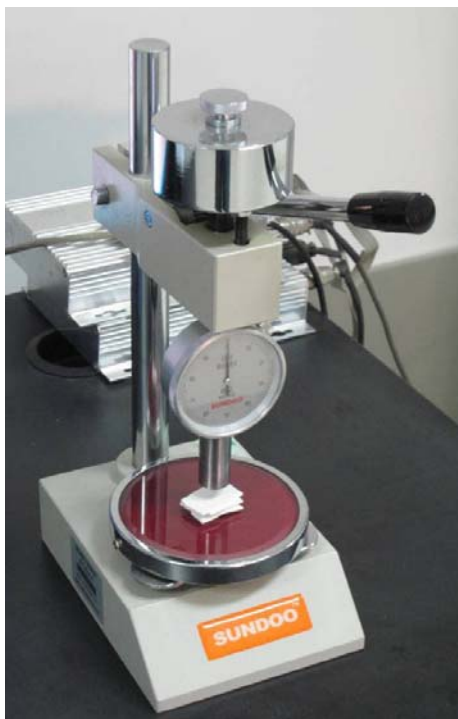
Figure 2: Shore A Hardness Testing of Sealant
